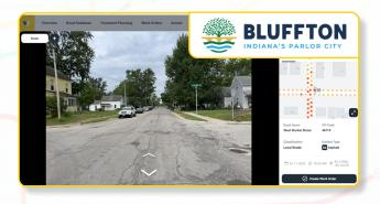
By entering real project cost data into the platform, Bluffton can instantly see budget scenarios for individual road segments. With measurements automatically captured from the smartphone-mounted assessment, they now generate cost estimates in minutes instead of days.
